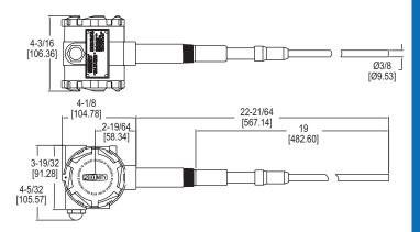
The Series CLS2 Capacitive Level Switch is a capacitive technology level switch which can be used for liquids, powders and bulk materials. It is offered with PVDF and 316 SS wetted material, weatherproof enclosure, DPDT output and a variety of process connections
