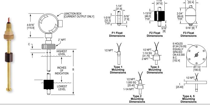
The SERIES CLT Continuous Level Transmitter provides up to the minute tank level monitoring with a customized level transmitter. Transmitters can be configured for 4 to 20 mA or proportional voltage output, 316 SS or Buna-N stem and floats, and lengths up to 72" (183 cm).
