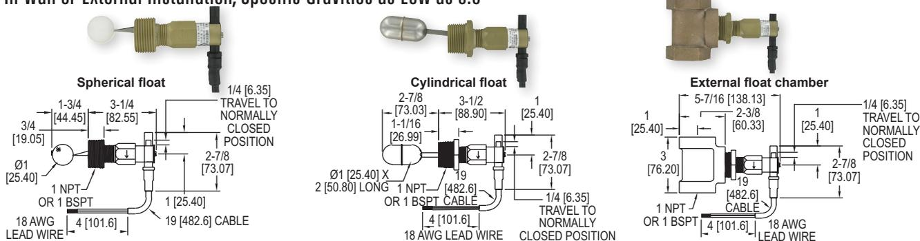
The **Series L10 FloTECT® Mini-Size Float Switch** is a series of economical, compact liquid level floats. It is offered in brass or 303 SS bodies and external tees as well as polypropylene or 304 SS floats with 1" NPT male threads, for direct side mounting through a half coupling, or with factory installed tee for external mounting. This series can be used in liquids with specific gravities as low as 0.5.
