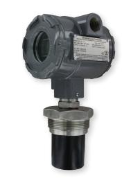
The **Series ULT Ultrasonic Level Transmitter** provides non-contact measurement of liquid levels in an explosion-proof body. It is capable of measuring up to 32.8' (10 m) with a PVDF sensor and 4-20 mA output.
